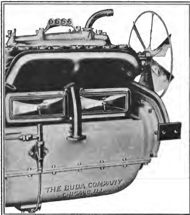
View of the right side of the Buda motor used in the new Tribune car, showing valve cover plates and manifold
